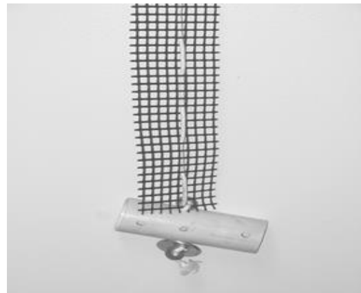
Figure 2. Image of a “Portland Sampler” substrate (Portland State University Center for Lakes & Reservoirs).
